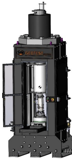
Cell Base Inserted into Load Frame
